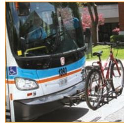
**2** To unload, pull the support arm out and down over the tire to release it.
