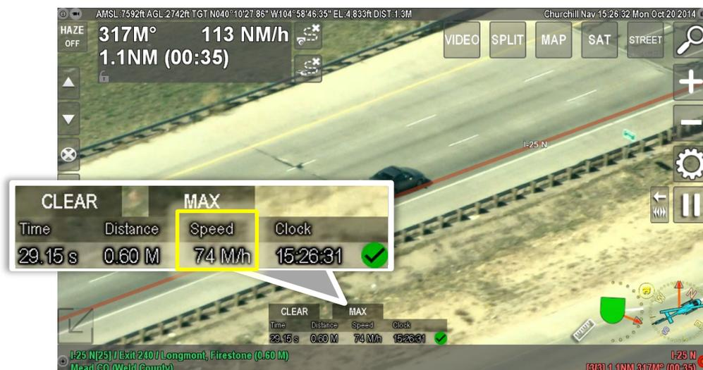
In this example, the vehicle was moving at least 74 mph over the measured distance (.60 miles) and time (29.15 sec).
