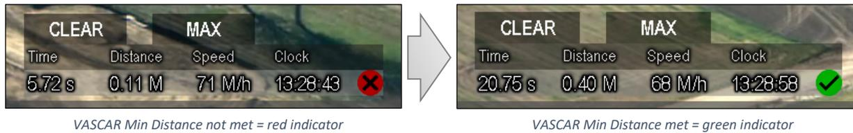
Once the tracked vehicle has travelled far enough to exceed the VASCAR minimum distance setting (usually one quarter of a mile), the indicator on the speed measurement window will turn from red to green indicating that the measurement process now has enough distance to return data with at least 95% certainty.
