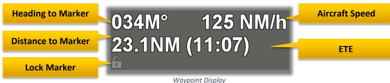
Select **On w/Arrow to** show the waypoint display with an on-screen arrow/overhead compass showing direction to the active marker as well as the azimuth where the camera is pointed.
