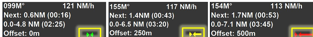
Note the Course Deviation Indicator in the bottom right of the Waypoint Display. The CDI changes from Green, to Yellow, to Red based on the Vehicle or Camera's offset relative to the Dynamic Layer's position.
