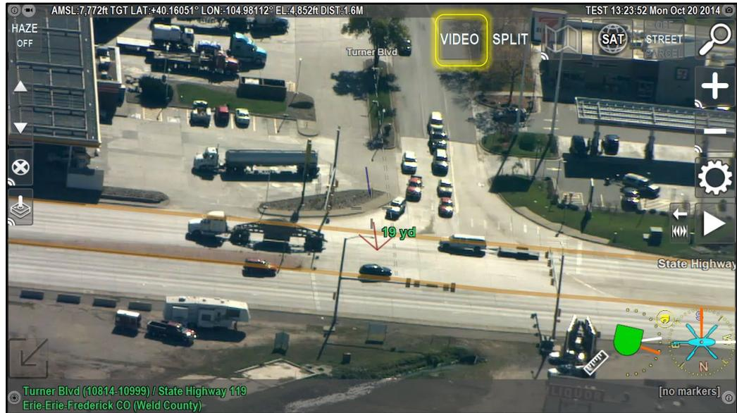
Pressing the on-screen **VIDEO** button (**F1**) enters Video Mode displaying real-time video with ARS's configurable overlay data.
