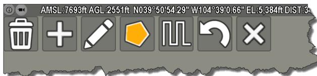
Create New Layer displays the layer menu in the upper left corner of the screen. Creating a custom layer auto-adds the layer to the Dynamic Layers menu with a default *yyyy-mm-dd-time* title. Selecting a layer in the Dynamic Layers menu displays the following options:
