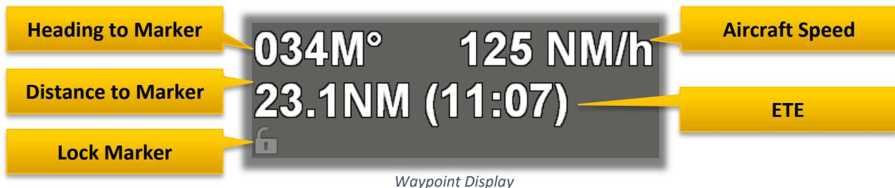
Selecting *On w/Arrow* shows the waypoint display with an on-screen arrow and overhead compass displaying the direction to the active marker as well as the azimuth where the camera is pointing.
