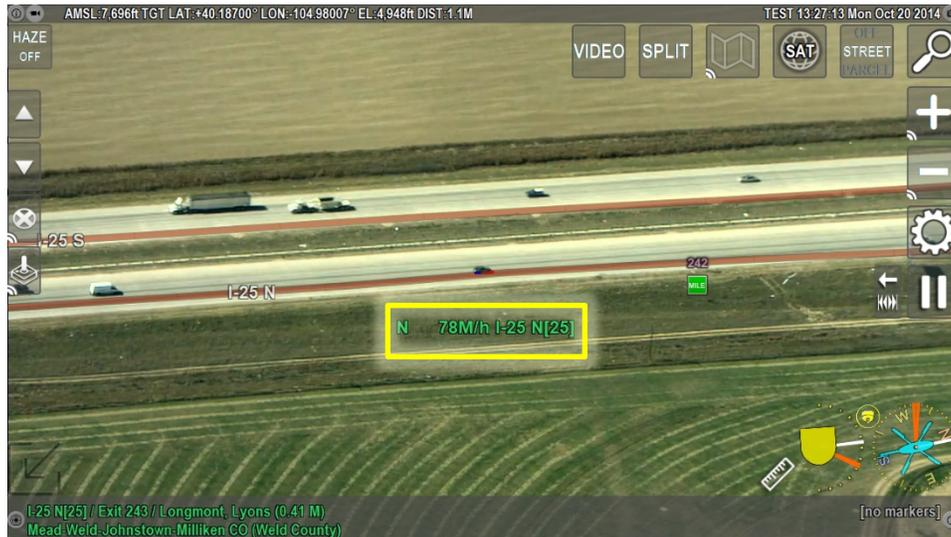
The North Indicator's display with Show Street set to Always. Note that highway I-25 is displayed next to the North Indicator's heading and speed.
