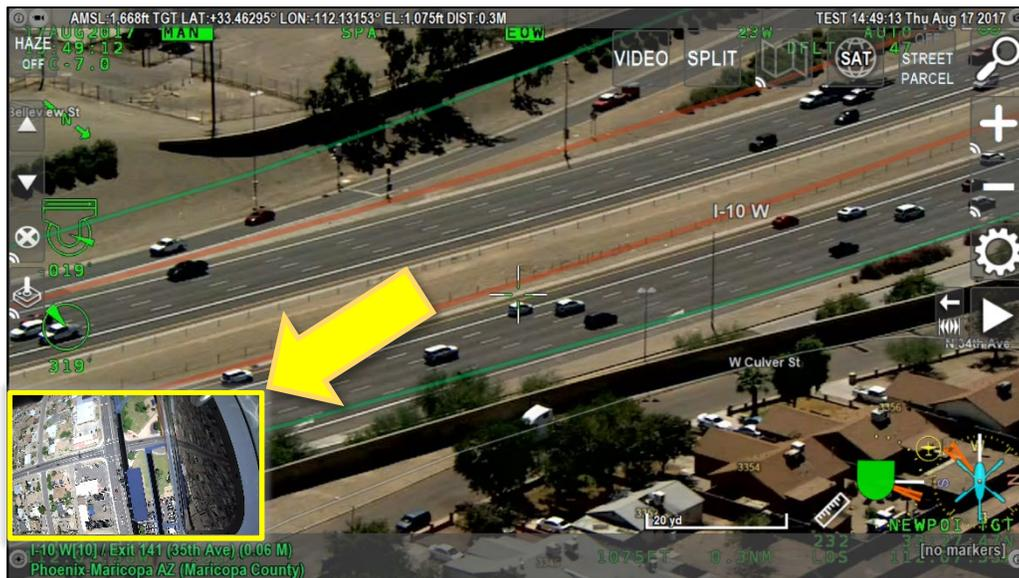
PIP simultaneously displaying the camera target and hoist camera.
